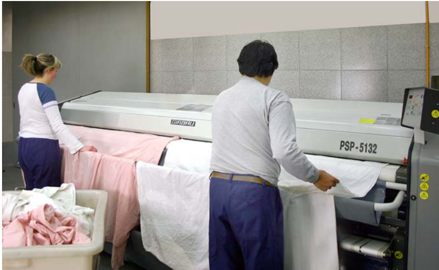
Girbau PSP-5132 flatwork ironer in operation
